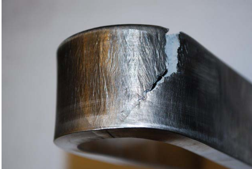
Photograph of a side-bend sample, which failed as a result of lack of fusion
