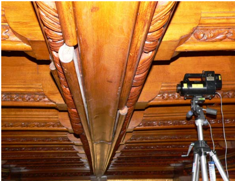
Figure 5. X-ray source positioned to take an image through the lower truss chord
