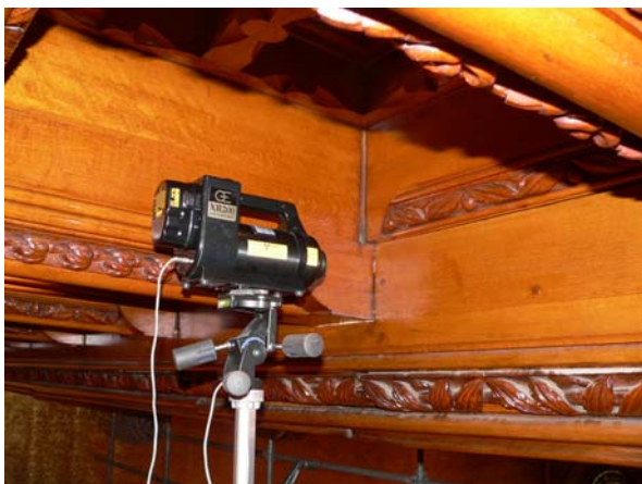
Figure 6. X-ray source positioned to take exposure #15
