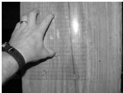
Fig. 9. The use of a  $\frac{1}{2}$ -inch grid on acetate for measuring slope of grain.
