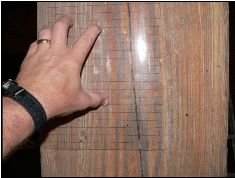
Figure 7. The use of a \frac{1}{2} -inch grid on acetate for measuring slope of grain on a post and timber. This slope of grain is 0.8:10, or approximately 1:12.
